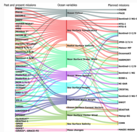
Figure 2: Sankey diagram linking past, present and future satellite missions and their sea ice measurement capabilities. (left) Past (identified with *) and present missions; (center) retrieved ocean variables; (right) future approved missions. RCM stands for RadarSat Constellation Mission.
